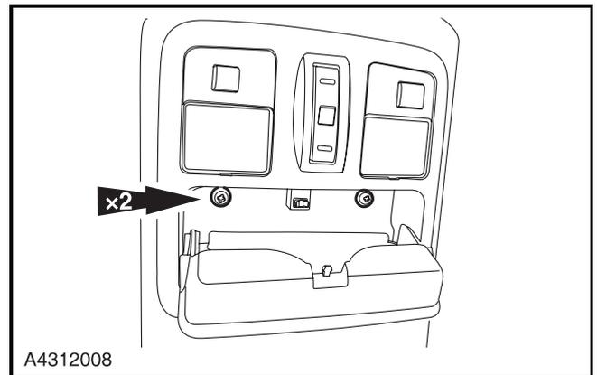
3. Detach the sunroof switch from the roof lining.
