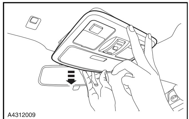
4. Disconnect the wiring harness connector of the sunroof switch.
