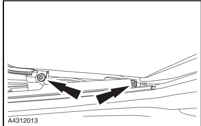
2. Remove the 2 retaining bolts of the sunroof glass.
